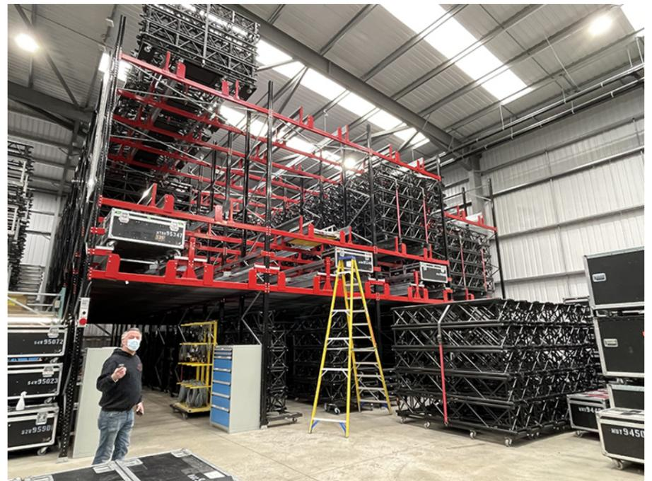
Ground floor picking levels allow for rapid picking of fast-moving products, contributing towards a significant operational cost saving. The design made use of readily available componentry from blue-chip suppliers, so parts could be replaced easily.
