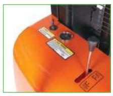
Key, Battery Life Indicator & the Fork Operating Lever on the Semi Electric Stacker
