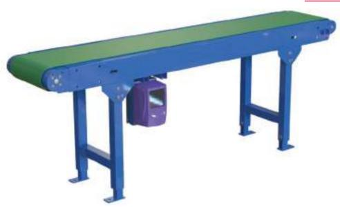
Motorised drum drive belt conveyor ideal for warehousing & light industrial use. Smooth faced anti-static PVC belt, supplied with variable speed controller with forward & reverse function. Rated at 30kg per running metre uniformly distributed load. Runs from a 230V (single phase) supply.
